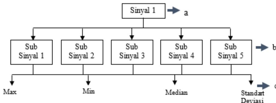
**Figure 3. Metode Teknik sampling, (a) Sample Sinyal, (b) Sample Sub Sinyal, (c)Seleksi Fitur**
