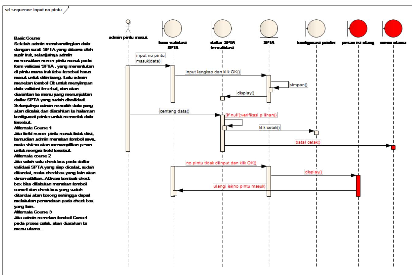
Figure 7. Diagram sequence input nomer pintu masuk
